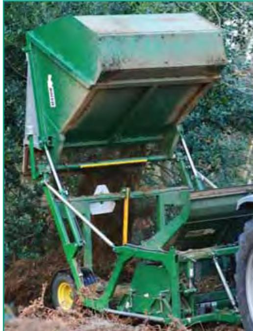
**Photo 6: New cut and collect mower:** This is a heavy flail cut and collect mower which is small enough to be attached to the back of the Council's compact tractor for use by the Rangers on the common. A trial has already taken place and discussions are currently ongoing for a planned purchase later in 2012.
